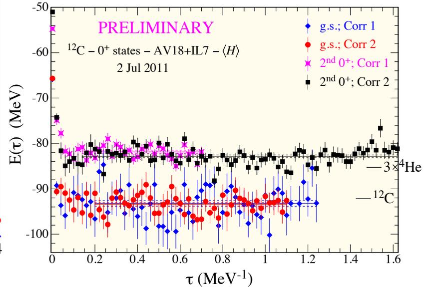
The ADLB (Asynchronous Dynamic Load-Balancing) version of GFMC was used to make calculations of  $^{12}\text{C}$  with a complete Hamiltonian (two- and three-nucleon potential AV18+IL7) on **32,000 processors** of the Argonne BGP. These are believed to be the best converged ab initio calculations of  $^{12}\text{C}$  ever made. **The computed binding energy is 93.5(6) MeV compared to the experimental value of 92.16 MeV and the point rms radius is 2.35 fm vs 2.33 from experiment.**
