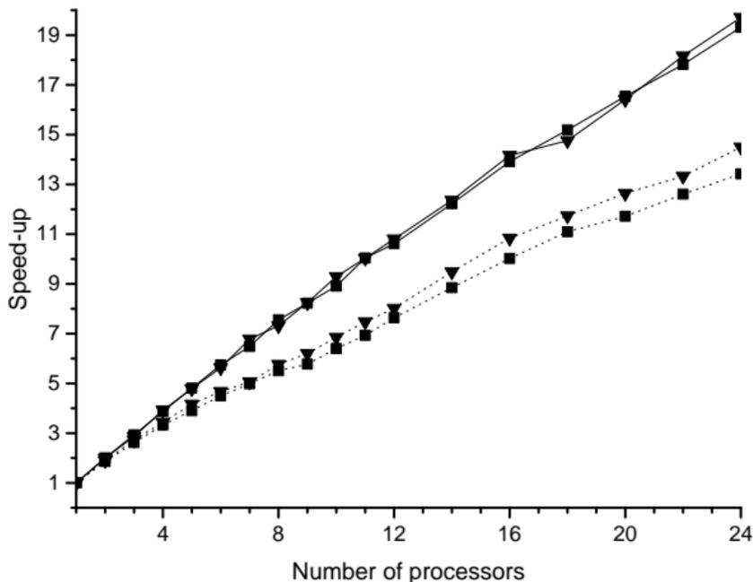
**Figure:** Calculation speed-up as a function of the number of processors. The squares and triangles are the results for the FEM degree of 7 and 9, respectively. The solid line corresponds to the matrix elements of the Hamiltonian, and the dot line does to the r.h.s.
