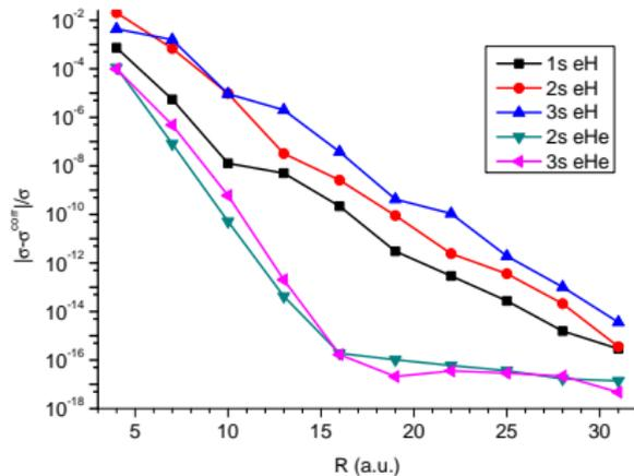
**Figure:** The relative difference  $|\sigma - \sigma^{\text{corr}}|/\sigma$  for the  $1s \rightarrow ns$  cross sections for the Temkin-Poet model as a function of the splitting radius  $R$ . The energy  $E=0.147$  a.u. above the ionization threshold, the ECS radius  $Q=121$  a.u.
